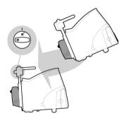
2. Slide the handle of the lower pump into the slot at the bottom of the top pump.
