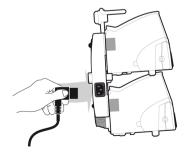
**4.** Insert the power cord into the black power socket on the side of the Agilia Duo.
