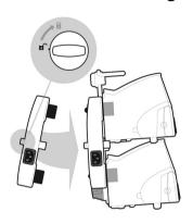
Insert the two black connectors of the Agilia Duo into the two black power sockets on the back of the connected pumps.
